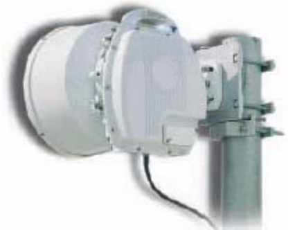
EX8500 Outdoor RF Unit (shown with integral antenna)
